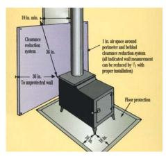
All combustible floors must be protected by non-combustible material extending eighteen (18") in front of the loading door. See diagram above for further detail.
